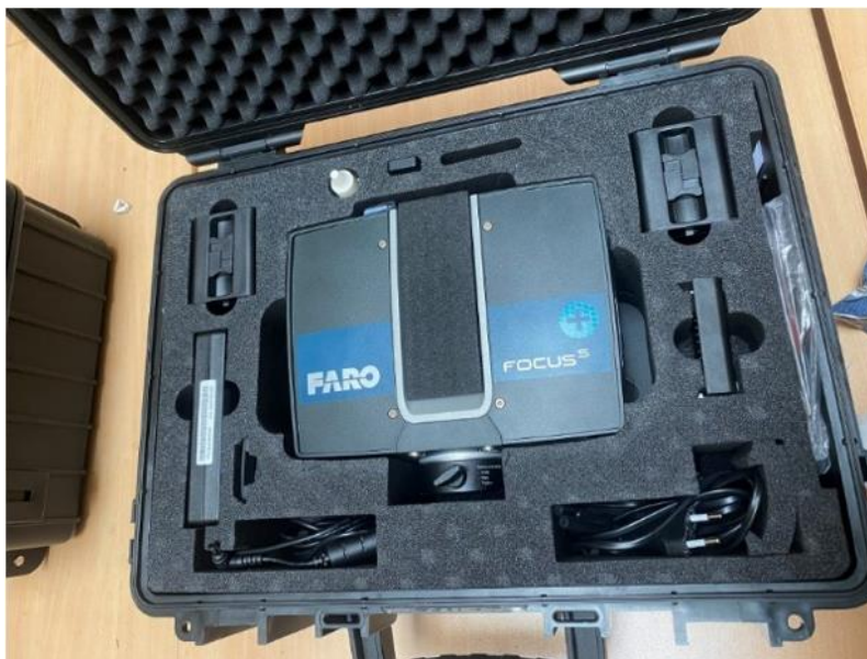
Figure 1. FARO Focus S+ 150 laser scanner.
